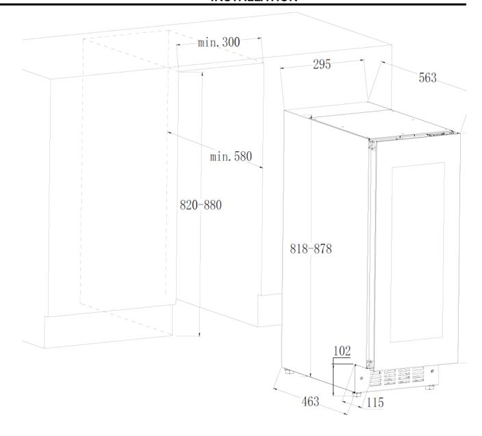
PLEASE NOTE - DIMENSIONS CAN VARY BY +/- 2mm DUE TO MANUFACTURING TOLERANCES, ALL DIMENSIONS ARE MILLIMETRES (mm)
